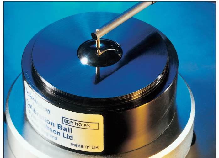
calibration over a ball checks stylus condition, gauge range, linearity and processor functions
